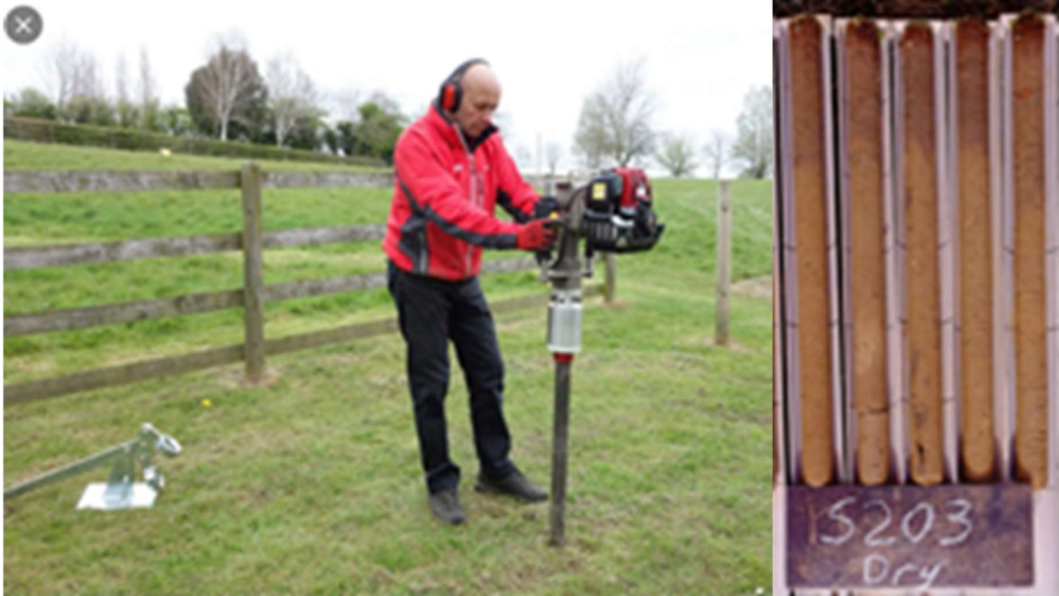
Figure 3. The hand-held mechanical corer method. A. Example of a hand-held 'vibrating' mechanical corer. At the left of the photo is the lever used to extract the core. B. Example of soil cores extracted from the sampling tube and placed into half pipes, ready for dissection into 10 cm increments.
