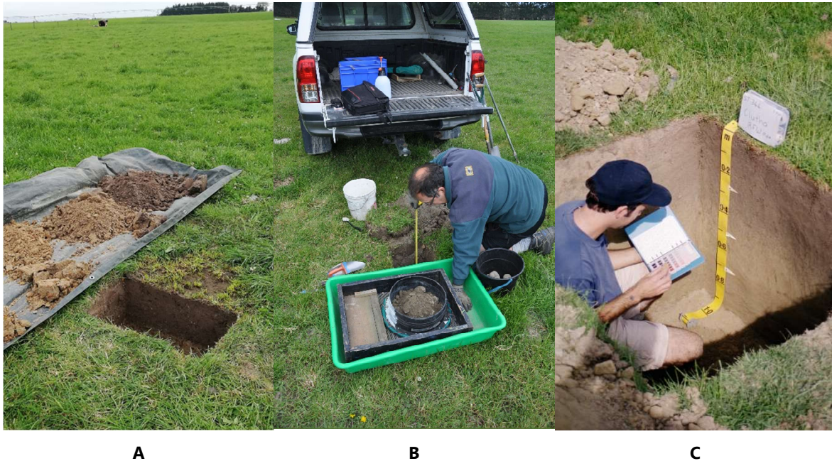
Figure 5. Examples of different soil pits for different purposes. A. A small, quick soil pit to identify key soil features. B. A small soil pit to measure stone content. C. A large soil pit to 1 m depth for full reference pit characterisation and collection of soil cores.
