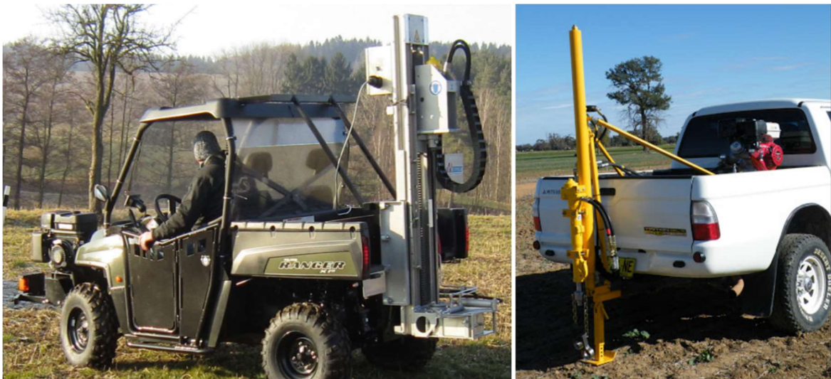
Figure 4. Vehicle-mounted mechanical corers. A. Hydraulic corer mounted on an ATV. B. Hydraulic corer that mounts on the deck and towbar of a 4WD ute.
