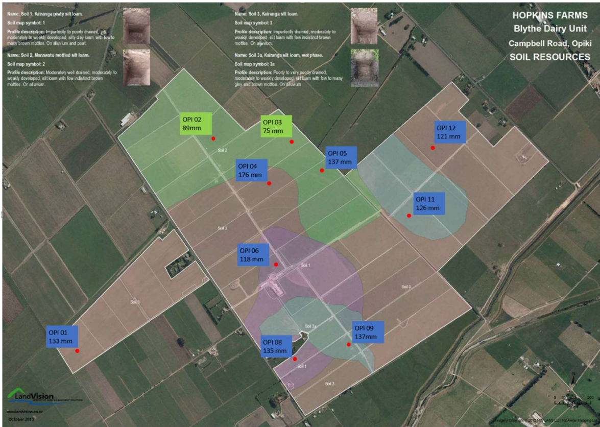
Figure 9. Observation sites on the Opiki farm in relation to the S-map soil map units, labelled by the site number and the AWC to 60 cm depth. Blue boxes indicate poorly drained soil, while green indicate imperfect drainage.
