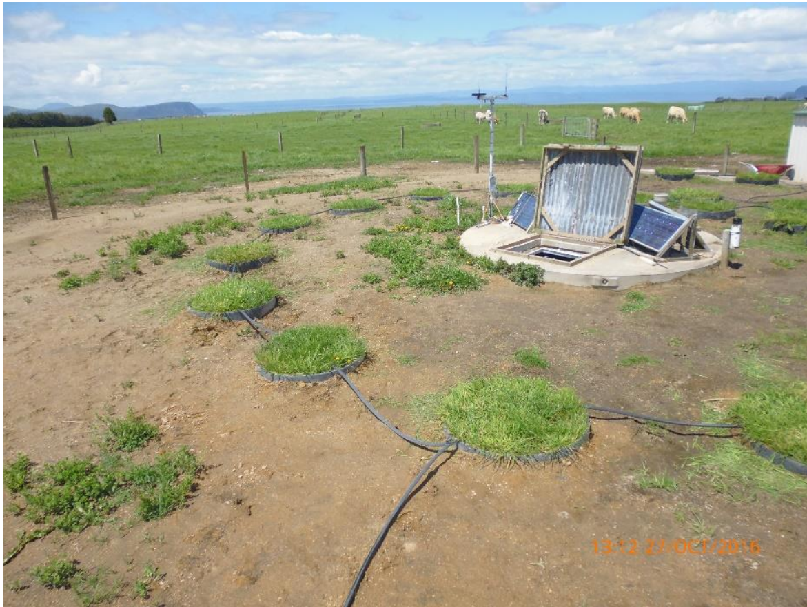
Figure 3. Farm stock water drip irrigation system used to flush any urine-N entrained within the soil column from grazing.
