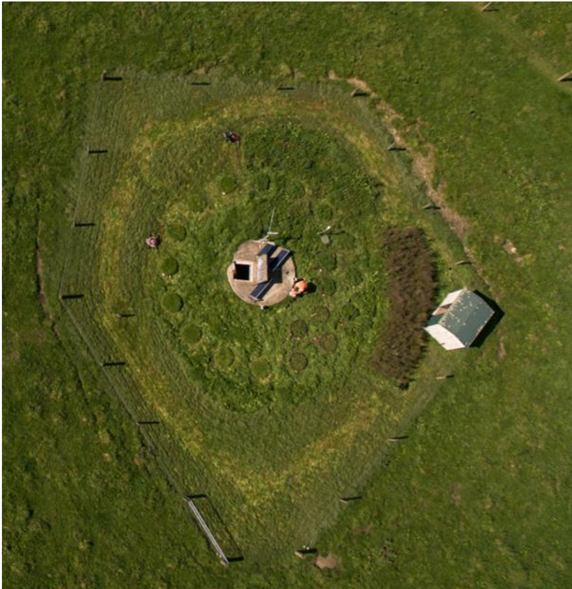
Figure 1. Aerial view of lysimeter facility at Tihoi. Pasture lysimeters and pasture guard crop are generally to the left of the central underground leachate collection facility, while lucerne lysimeters and guard crop are generally to the right. Immediately to the left of the shed are manuka lysimeters and guard crop not involved in the SFF study.
