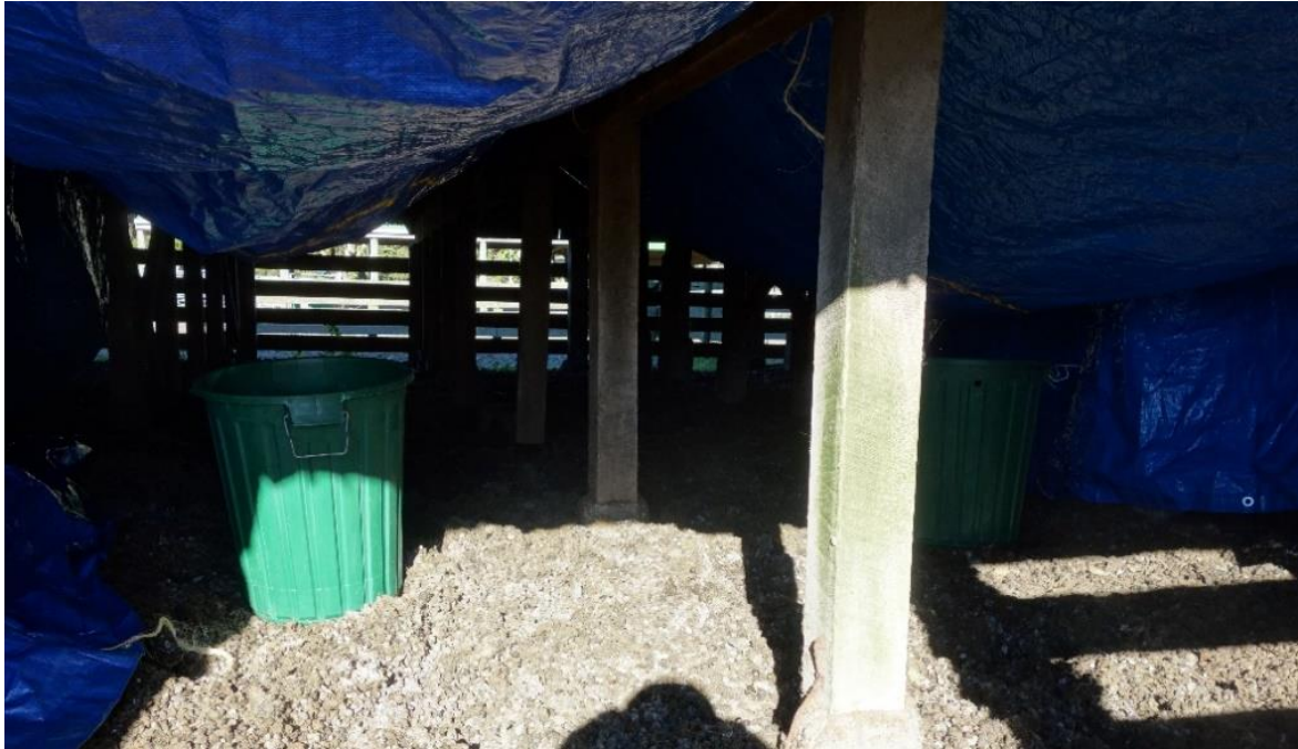
Figure 6. Ewe lamb urine being collected into 60-L vessels via plastic tarpaulins spread under the grating in a woolshed.
