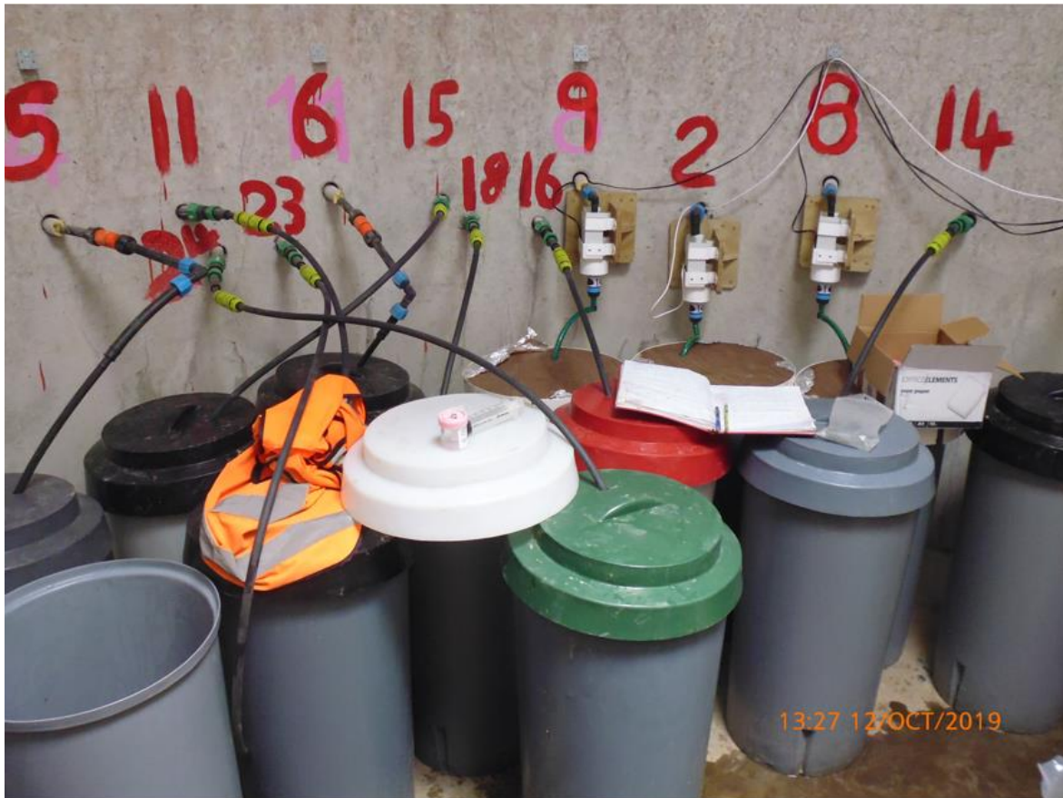
Figure 8. Leachate collection barrels in the underground facility. Numbers on the wall indicate lysimeter number. Lysimeters 16, 18, 23, and 24 grow a separate crop and are not part of this study. Under some lysimeters, leachate passes via tipping bucket recording devices to monitor leachate volume.
